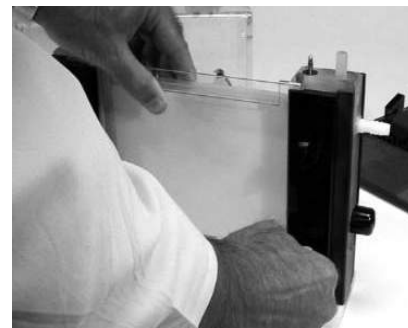
Figure 4-5. Tighten Wing Knobs
