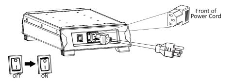
After connecting the power cord, switch ON the mains and switch ON the stirrer from rear side as shown in above image.
