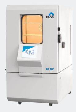
The ID 301 Climatic Test Cabinet has been developed to revive natural climatic conditions. The wide temperature and humidity control range of ID 301 allows many products to be tested in different climatic conditions, and stability, artificial aging and shelf-life tests can also be easily carried out.
