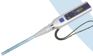
L-7 (integrated) Introduction of a small, handheld pH meter with integrated electrode.
