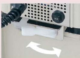
Bath can be dismantled by lever rotation.
