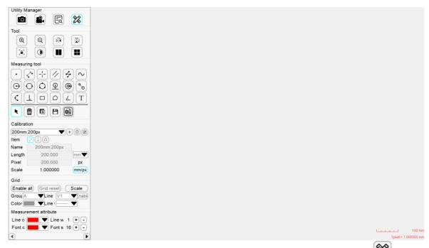
To activate the measurement function, click on the measurement icon in the Utility Manager. The system offers up to 20 different measurement types.
