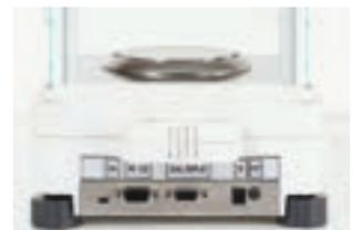
Features RS 232 communication, allowing for error-free documentation, ensuring accurate and reliable data transfer Pc or printer.
