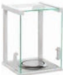
Designed with a spacious glass draft shield 3 side opening and an IP54 protection class for efficient and safe operation, and protection against dust and water splashes.
