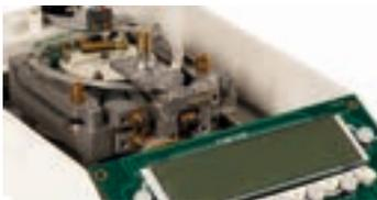
The Mono-Tech technology sensor truly stands out with its unparalleled design based on electromagnetic force compensation (EMFC). Its exceptional performance meets the highest international standards. I am truly impressed by its unique features and the results it delivers.
