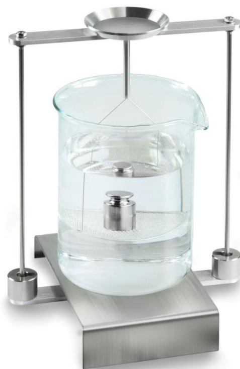
Figure 2: Weighing in auxiliary liquid
