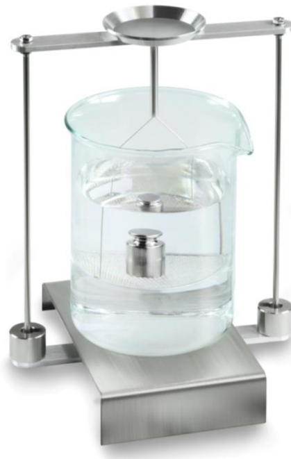
Fig. 2: “Weighing in test liquid”
