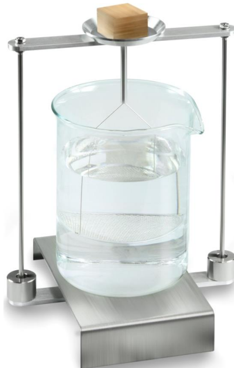
Fig. 3: Weighing in air
