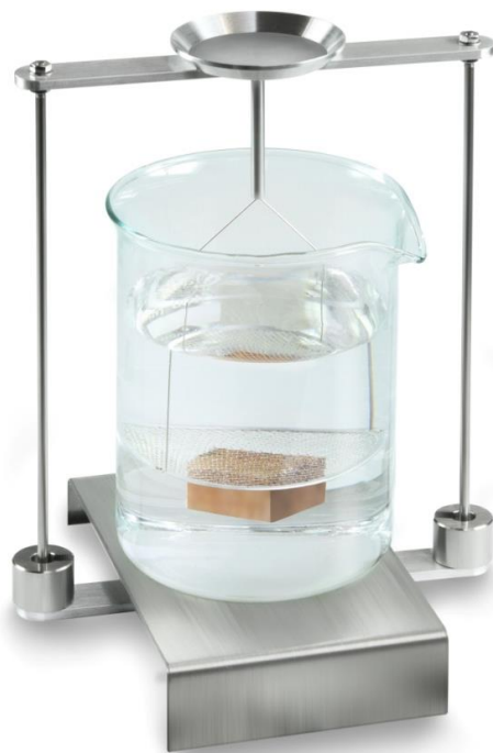
Fig. 4: Weighing in the auxiliary liquid
