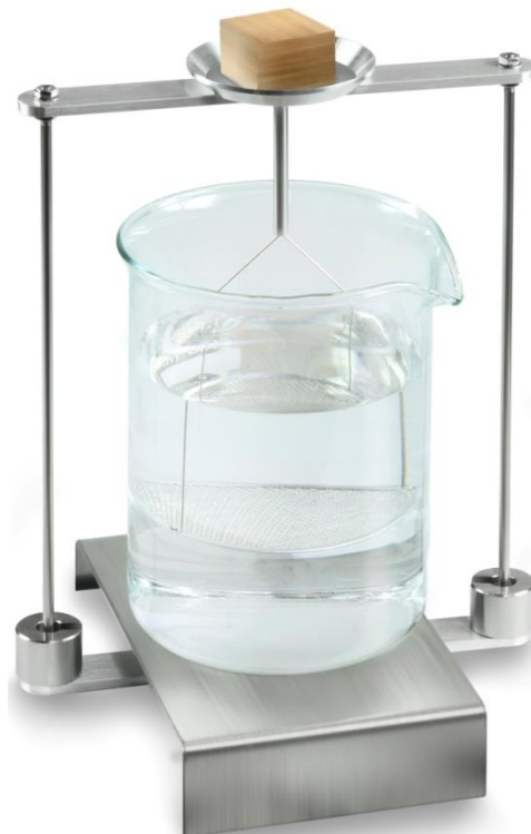
Fig. 3: Weighing in air
