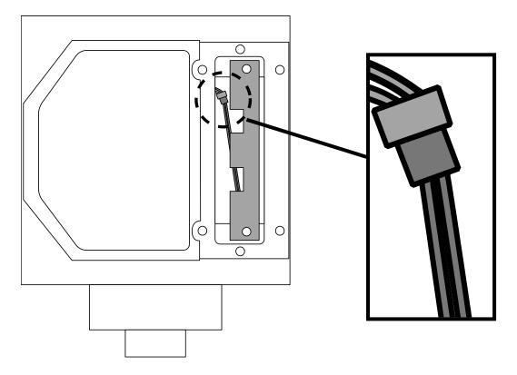
6. Fasten the rechargeable battery pack using the delivered screws and washers.
