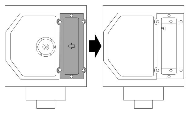
5. Insert rechargeable battery pack and connect with the plug.
