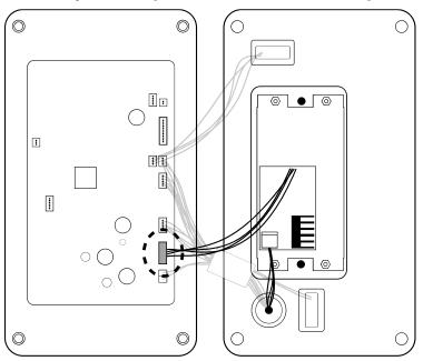
14. Fasten the rear side of the housing again with the four screws (see step 2)
