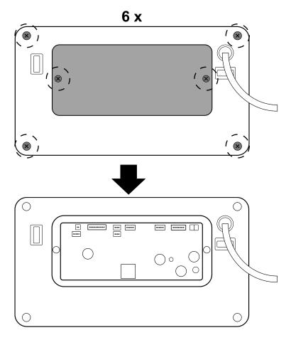
3. Carefully detach the back of the terminal from the front.
