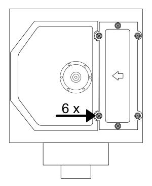
**4.** Remove the battery compartment cover.
