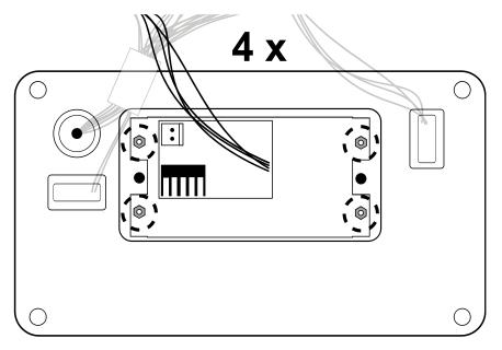
10. Connect the power supply to the control unit.
