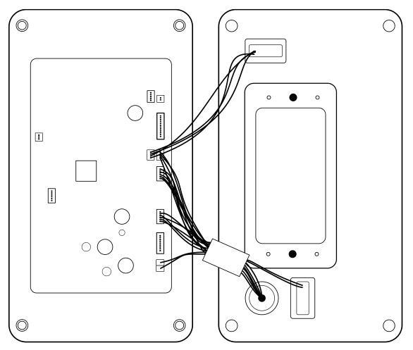
4. Clean the inside of the back of the housing with rubbing alcohol.
