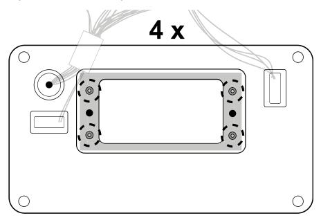
7. Place the control unit with the holes on the screw pins
