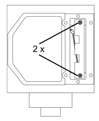
**7.** Fasten the battery compartment cover again with the screws (see step 3). The arrow of the cover should point to the center of the platform.
