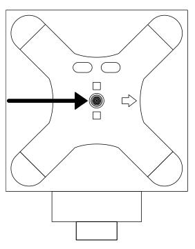
3. Remove screws and washers of the battery compartment cover.
