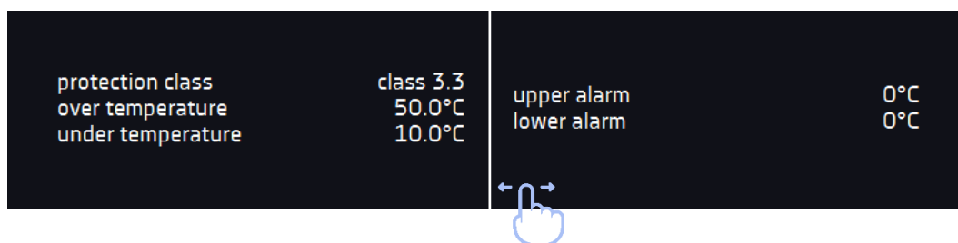
Figure 13 Status – protection and alarms
