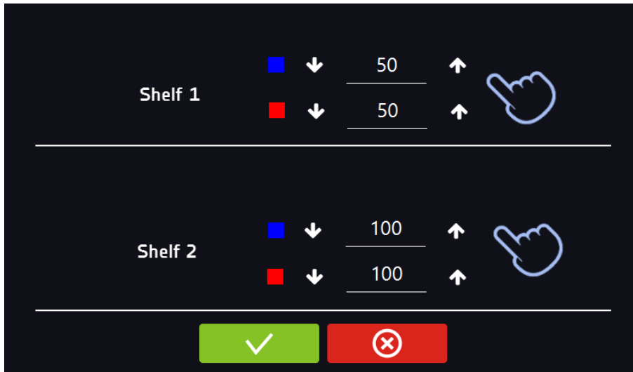
Figure 30 Setting the light intensity in active panels
