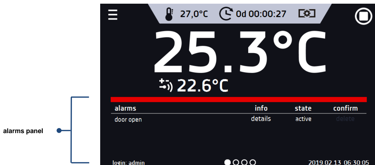
Figure 10 Icon: Alarms panel
