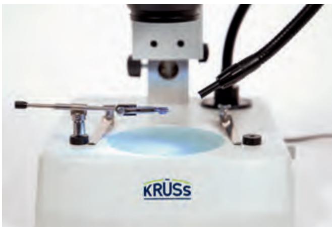
Figs.38a (left) and 38b: Using an incident-light device on the basis of dark-field microscopy and schematic depiction of this illumination
