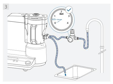
Hose recommendation:  $\varnothing$  6.0 (inside diameter) x 1.5 mm. Max. permissible pressure in cooling circuit 0.5 bar.
