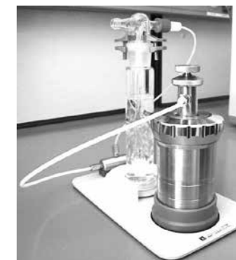
Venting using the Venting Station C 7030
