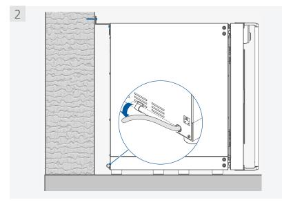
> Extend the drain hose with included hose adapter as necessary
