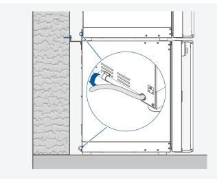
Extend the drain hose with included hose adapter as necessary
