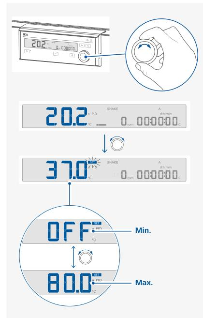
/// Setting the shaker speed / fan speed / light
