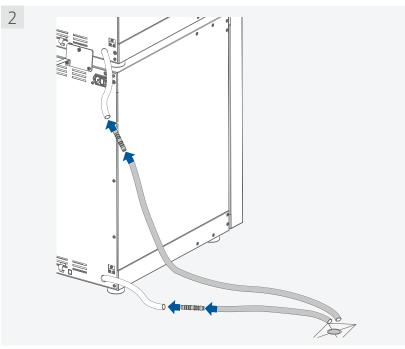
The devices drain hoses must be guided to the laboratory drain with the hose adapters and extension hoses.
