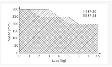
In order to ensure safe and secure operation, the shaker platform must only be operated within the range of usable weight and speed (see diagram - hatched area).
