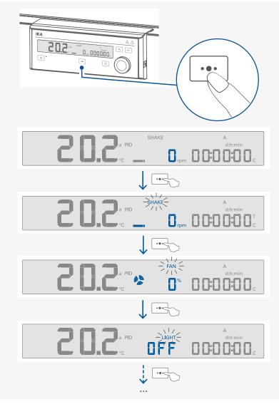
**Note:** Switching between the shaker / fan and light function by touching the multifunction button (F). The selected function blinks. Then, the value can be adjusted respectively by rotating the control knob (H).
