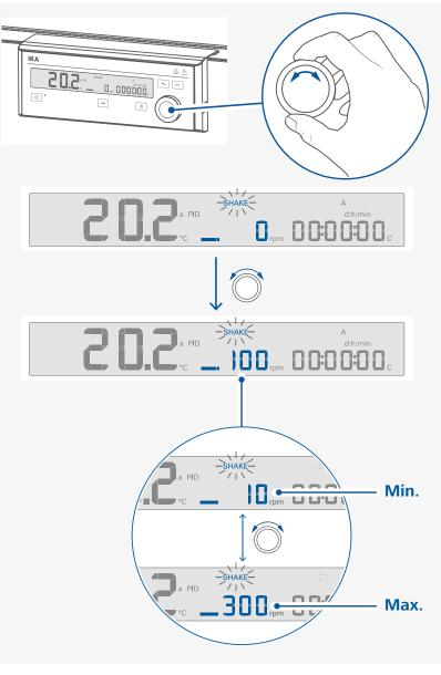
**Note:** When the device is running, the shaker speed can also be adjusted.
