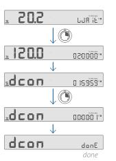
When the decontamination process is finished, the "dcon done" appear on the display. Press control knob to confirm it and screen back to "dcon off" as below:
