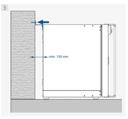
Note: The screws used for fixing is selected according to the wall conditions and is not included.
