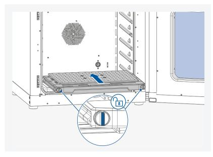
**Note:** When assembling the shaker platform, ensure the shaker platform locking knobs are turned to unlock status.
