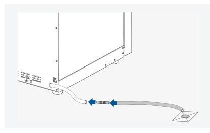
In the event of glass vessels breakage, the leaked liquid is collected by the drain pan (not included in delivery scope) below the shaker platform and is guided to the drain hose. Place the drain hose in laboratory drain.
