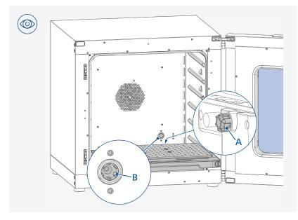
**Note:** When assembling the shaker platform, ensure the shaker platform coupling (A) is inserted into the coupling (B) correctly in the device.
