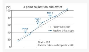
Individual load and ambient condition might influence the temperature behaviour of the chamber. To compensate that influence there's the option to neutralize by using the 3-point calibration and offset function. This function allows the temperature to be calibrated and adjusted at three different temperature values.
